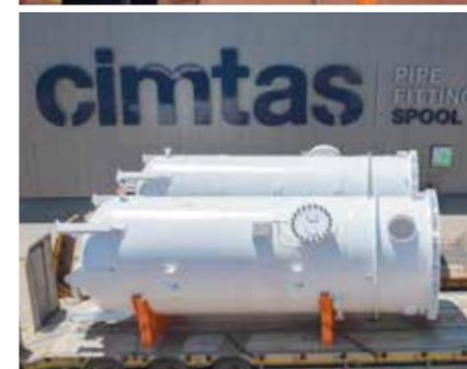
Engineering, design, procurement and fabrication of Pressure Vessels, Shell & Tube Heat Exchangers in accordance with ASME BPVC codes including U Stamp, EN 13445, TEMA where applicable, in various materials including HIC-tested carbon steel, alloy and low-alloy steel, clad (or weld-overlay) steel, vulcanized rubber lining and solid stainless steel.
