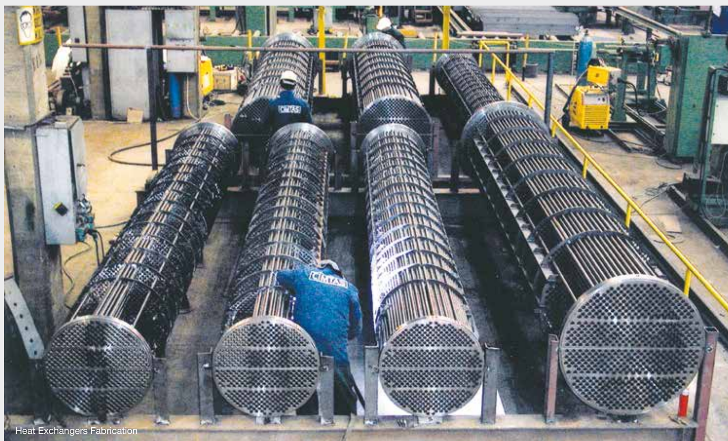
Vacuum Residue Coolers ID : 1,016 mm t : 13 mm/18 mm L : 7,455 mm W : 14 tons each
