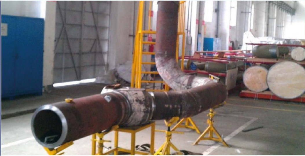
MAIN STEAM PIPING
