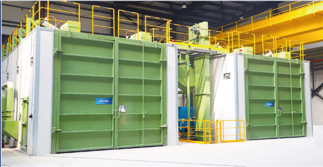
AUXILIARY EQUIPMENT GRIT BLASTING DIMENSIONS: 14.0x5.0x4.5m QUANTITY: 3 UNITS
