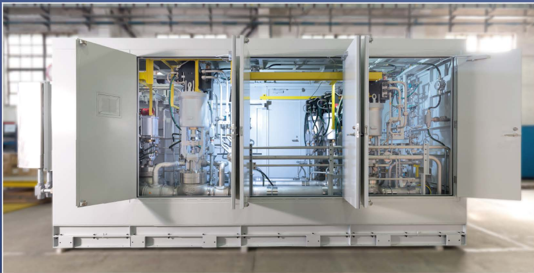
MITSUBISHI POWER M701 F4 FUEL GAS SKID
