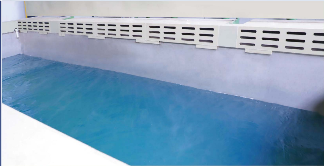
AUXILIARY EQUIPMENT PICKLING POOL
