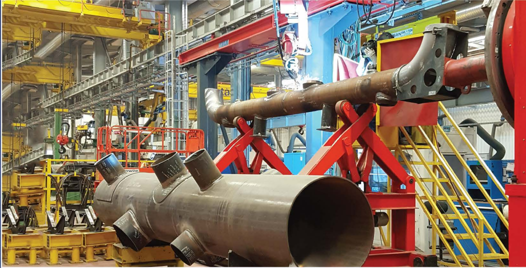
PIPE SPOOL FABRICATION
