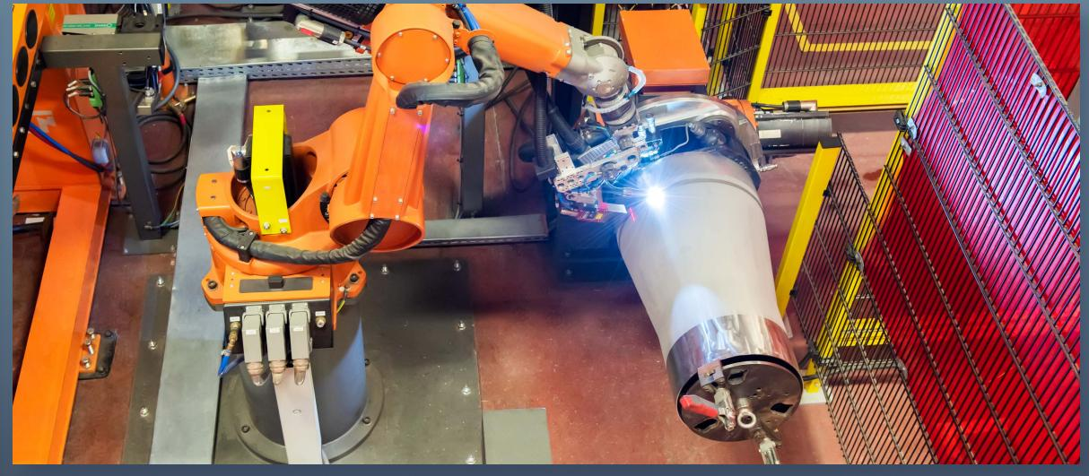
COLD METAL TRANSFER (CMT) ADDITIVE WELDING
