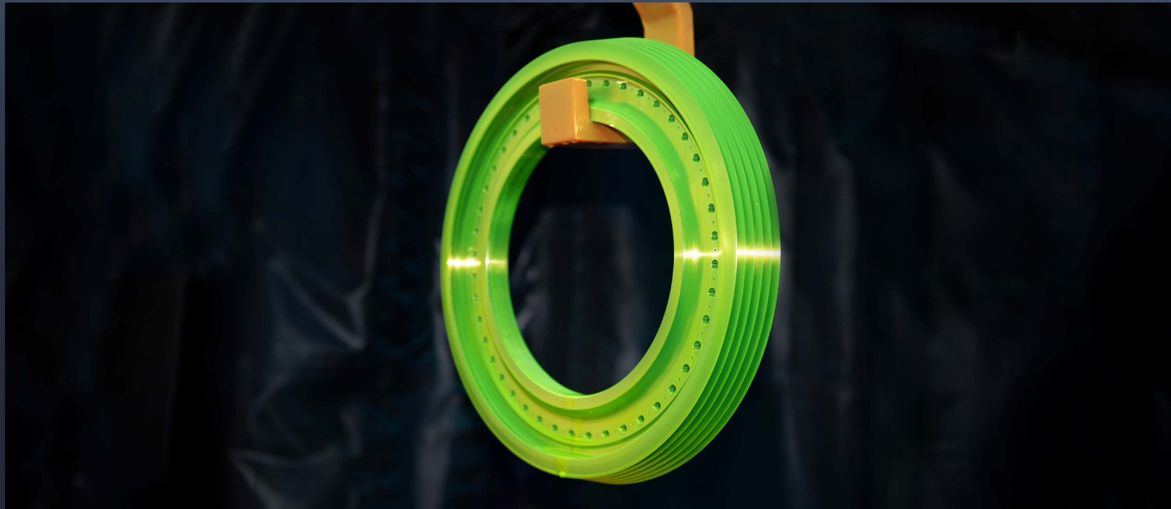
FLUORESCENT PENETRANT INSPECTION
