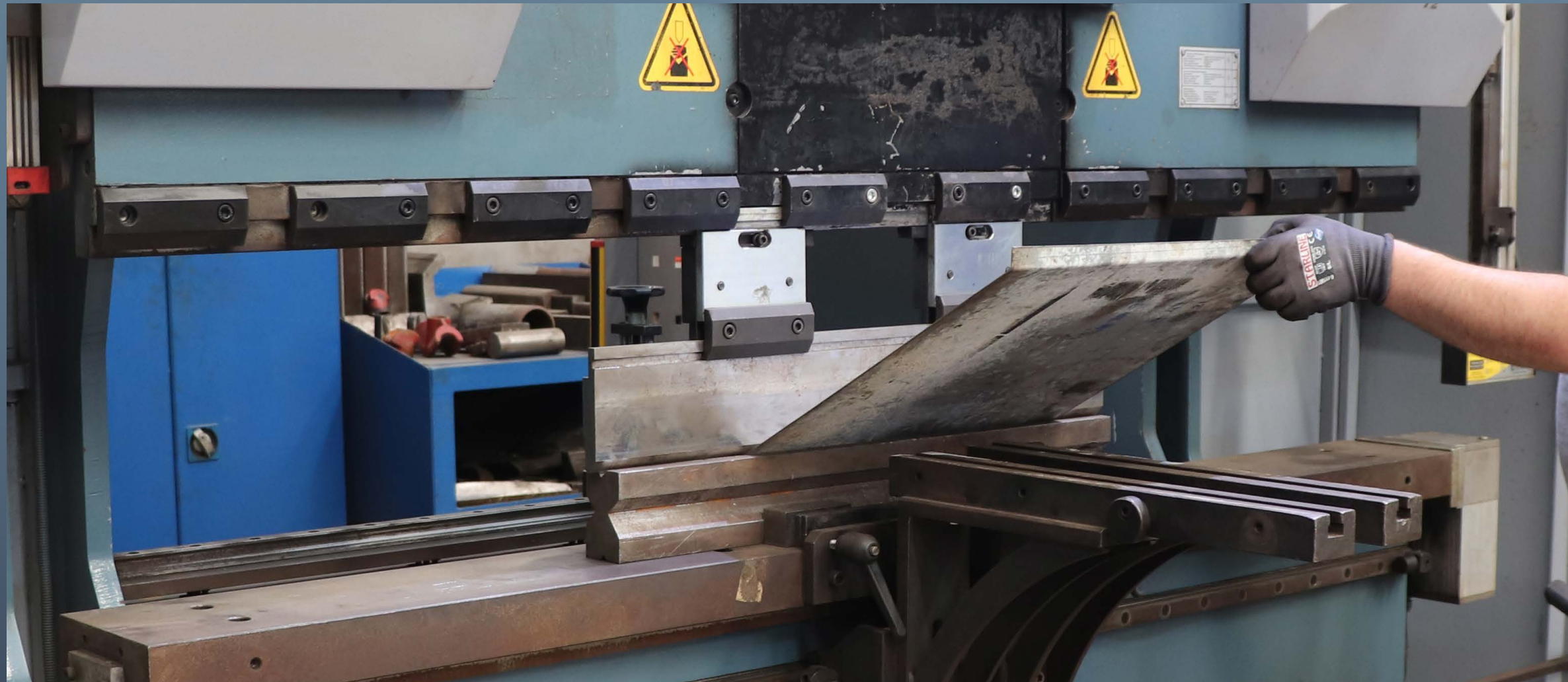
CNC PLATE BENDING
