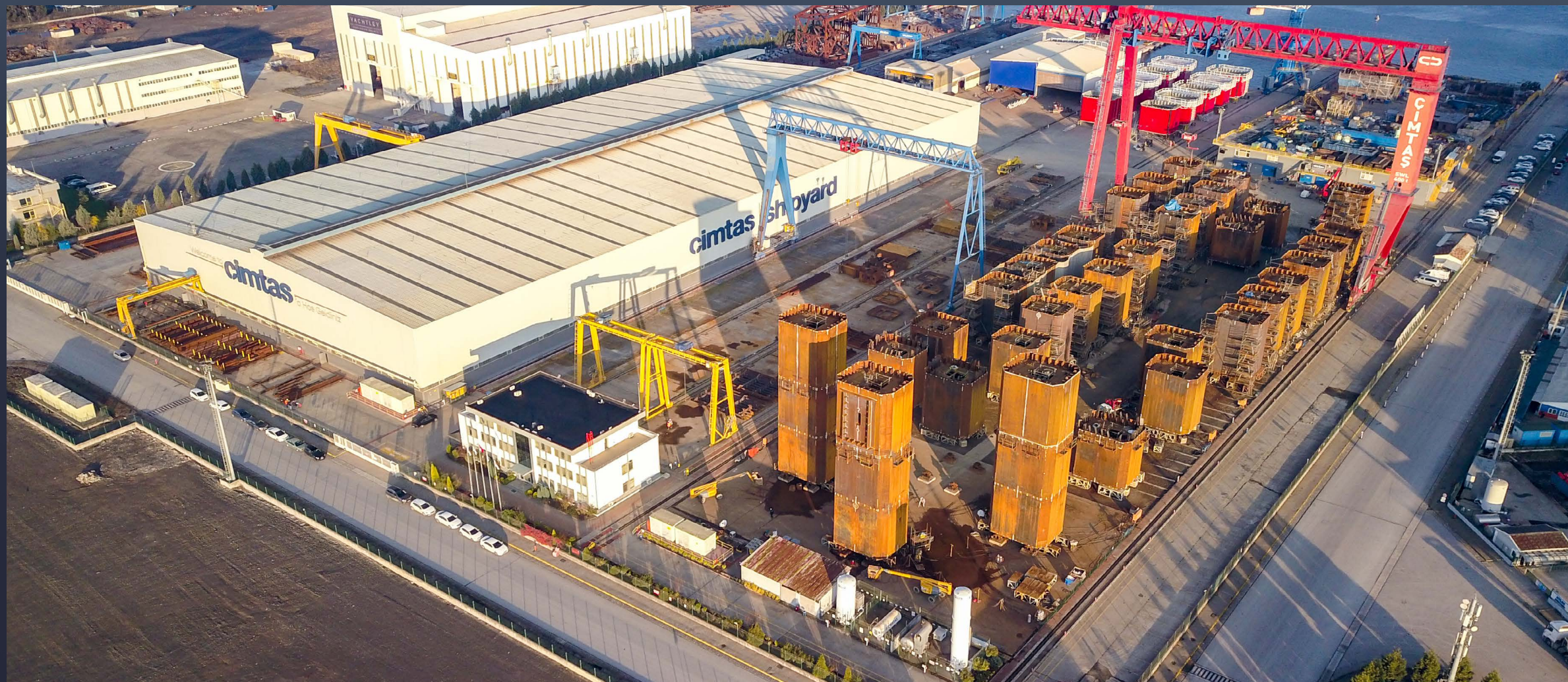
TOWER BLOCK FORMATION & TRIAL ASSEMBLY
