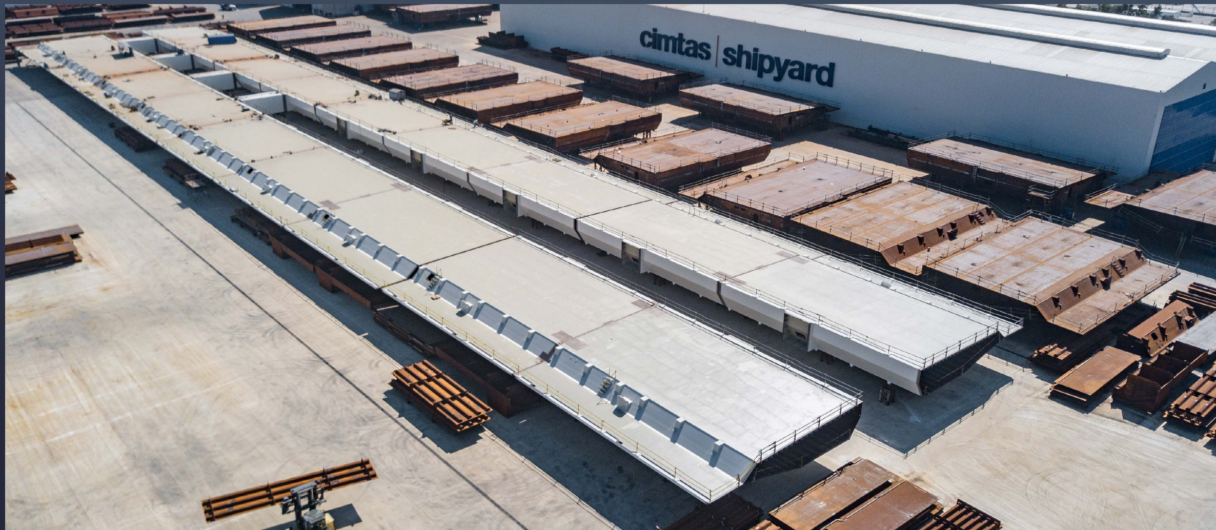
GIRDER BLOCK TRIAL ASSEMBLY
