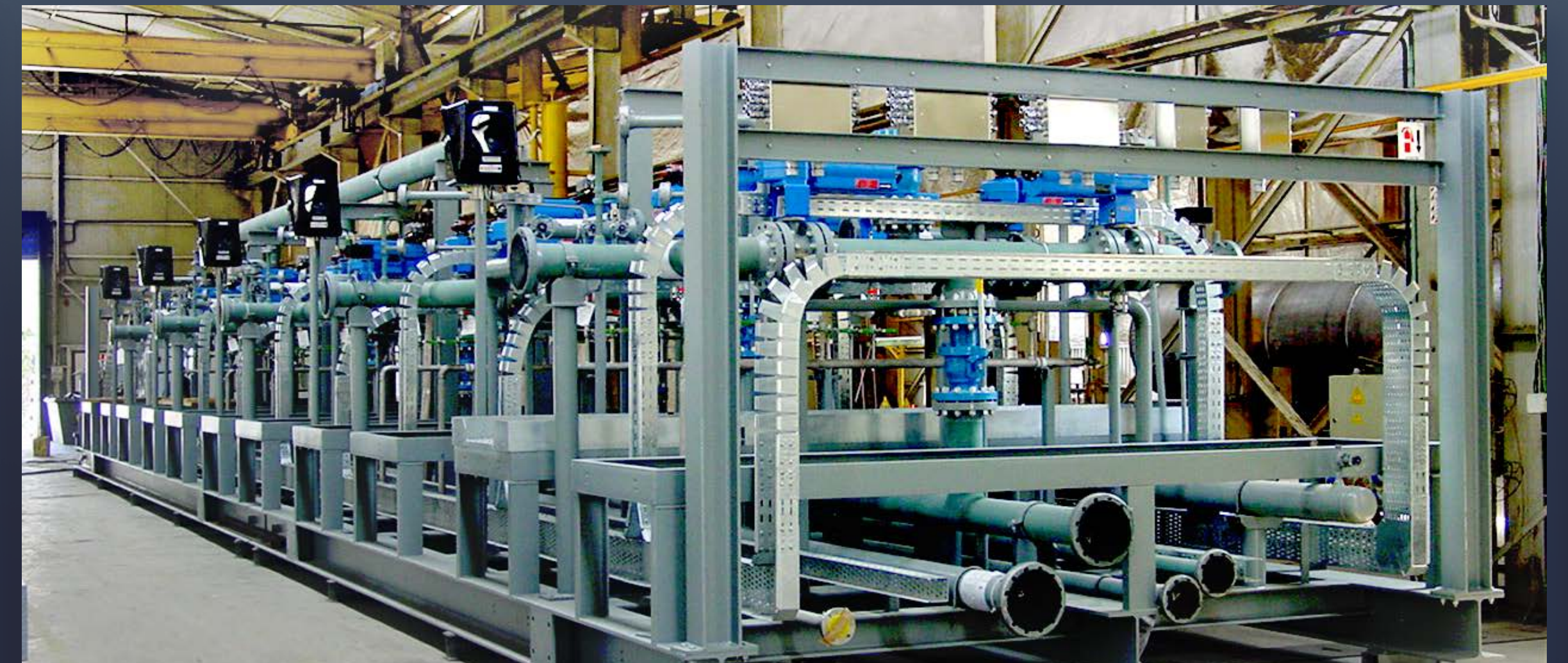
POLY BED HYDROGEN PURIFICATION SKID
